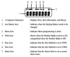
If the NOAA icon is ON but the TONE and VOICE icons are OFF, the Weather Receiver is available (ON) for listening to NWR broadcasts and the Alert Method is DISPLAY (Alerts will be displayed, but no Alert tones will be sounded).
